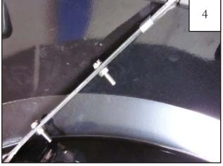
Insert the Screw/Washer assembly through the hole drilled in the end of the Front Main Flare and into the corresponding hole in the Front Bumper Piece. Two places. Install Clip CL1-0001 as close to outer edge as possible.
