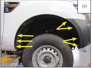
Using a Phillips Screwdriver and or pry tool, remove seven (7) factory screws/retainers from the wheel well and discard. *Note:* Some vehicle models will have factory mudflaps. These will need to be removed for proper installation of flares.
