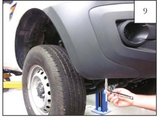
Using a 10mm socket remove One (1) factory bolt from under front bumper area of wheel well. Save factory bolt for reinstallation.
