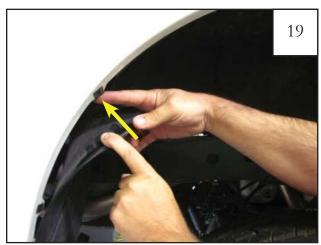
Peel back the rear wheel well liner and install one (1) supplied clip (CL1-0022) at the location indicated. Replace liner to original position.
