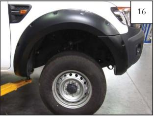
Tighten all screws. Front flare installation complete.
