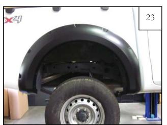
Tighten all screws. Rear flare installation complete.
