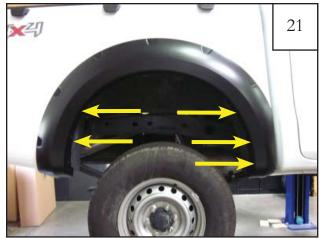
While holding Rear Flare onto vehicle using a #2 Phillips Screwdriver, start six (6) supplied Screws (SW1-0056) into flare and into clips installed in steps 17 & 18.
