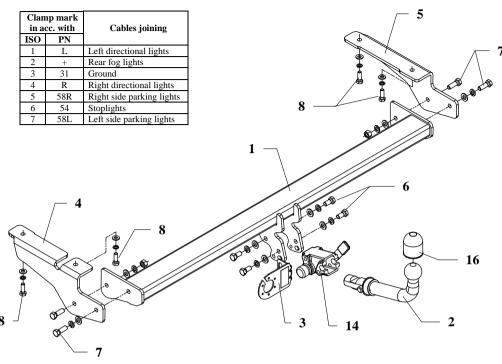
This towbar is designed to assembly in following cars: CITROEN C5 I, 4 doors, produced since 2000 till 09.2004, catalogue no. P24A and is prepared to tow trailers max total weight 1600 kg and max vertical mass 85 kg.
